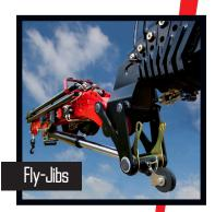
HMF provides different types of Fly-Jibs; It is possible to lead the winch via the Fly-Jib. HMF Fly-Jibs are available with extra valves, and this means that you can for example fit a grab on the Fly-Jib.
